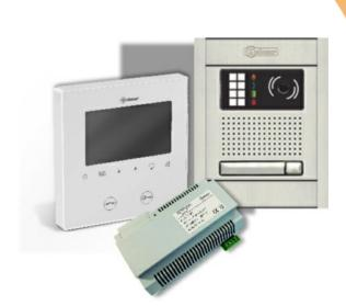
This kit has a 1.8 mm extruded aluminium door panel of modular design. Designed for ease of installation with internal modules connected through flat cables and pre-wired buttons. The information / camera window is manufactured in polycarbonate with steady illumination at the door panel through white LED's.
